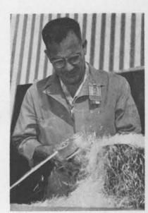
LIKE CAKE FROSTING, glass fibers spray from a hand-held chopper to a plastic-coated part. Alternating layers of fiberglas and plastic spray produce a strong fiberglas laminate. The chopper being used by Don Beard (8115-2) was developed by 8115 for this type operation.
